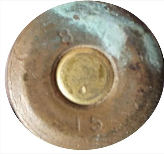
A circular brass ammunition headstamp with a central primer. The numbers "811" are stamped in the upper half and "15" in the lower half.  |
