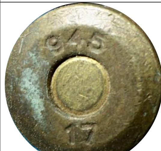
A circular brass ammunition headstamp with a central primer. The numbers "945" are stamped in the upper half and "17" in the lower half. |
