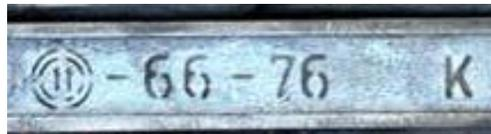
Stabilizer for strip propellant in 40 mm PG7 fin stabilized rocket propelled grenade, ammunition code 11-66-76 K indicating manufacture in Bulgaria in 1976
