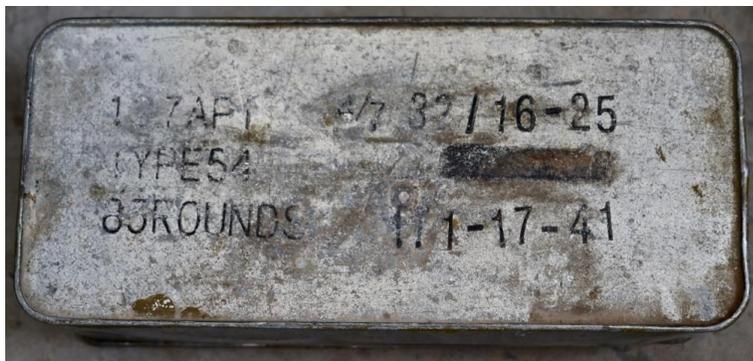
Figure 2: 12.7x108mm Armoured Piercing Incendiary (API) with marking: 12.7 API TYPE54 88 ROUNDS 4/7 32/16-25 112-17-41 (with characteristics similar to ammunition produced in China for Type54 weapons)
