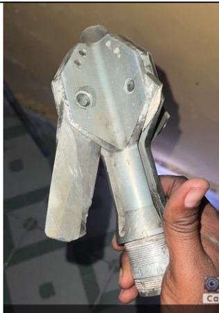
Fin stabilized rocket with retractable blade fins with characteristics similar to those of ammunition for 73 mm recoilless SPG 9
