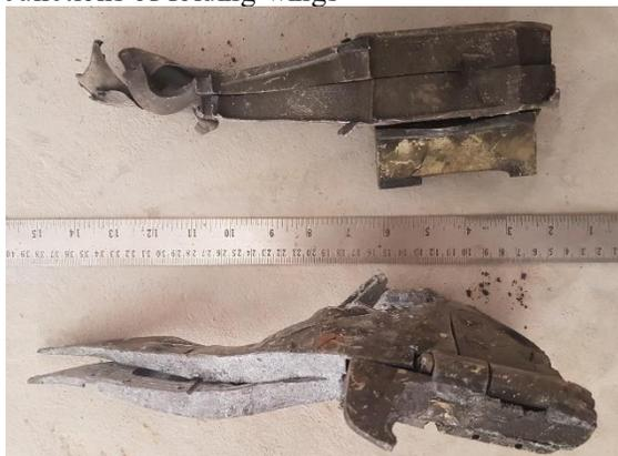
Compressor of a TRI-60 Microturbo engine
