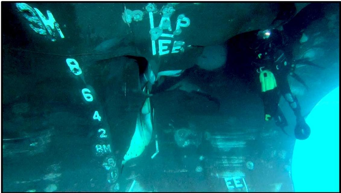
*Figure 11: Image depicting a diver in front of the damaged hull of the AL MARZOQAH*
