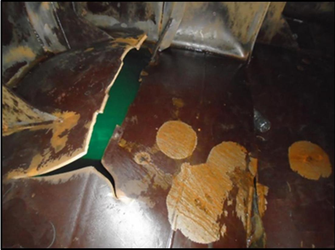
*Figure 12: Damage to the floor of the engine chamber sustained by the AL MARZOQAH*
