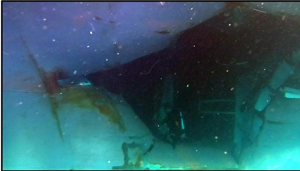
*Figure 2: Image depicting a diver in front of the damaged hull of the AMJAD*
