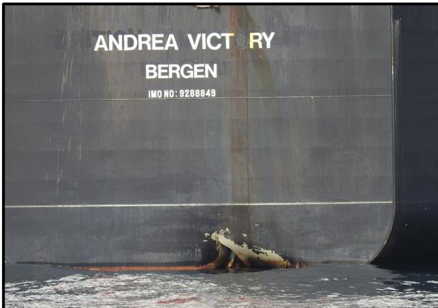
*Figure 20: Exterior of the ANDREA VICTORY, depicting the damage to the hull of the vessel*
