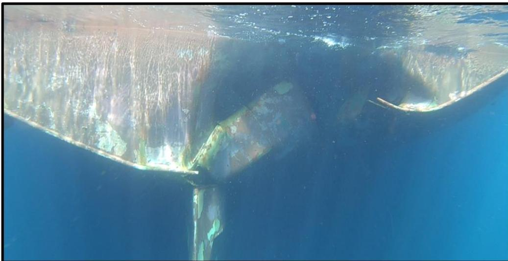
*Figure 21: Hull damage sustained by the ANDREA VICTORY*
