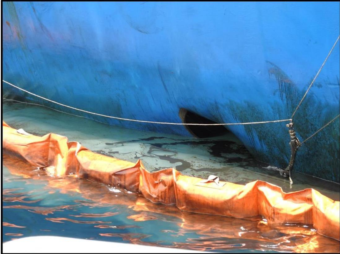
*Figure 15: Exterior of the A.MICHEL, depicting the damage to the hull of the vessel*
