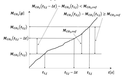
The duration  $(t_{2,j} - t_{1,j})$  of the j<sup>th</sup> averaging window is determined by:
