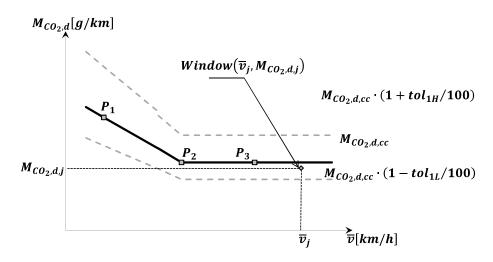
$Figure\ A8/4-2$  Vehicle CO<sub>2</sub> characteristic curve and tolerances for OVC-HEV vehicles for 3-phase WLTP
