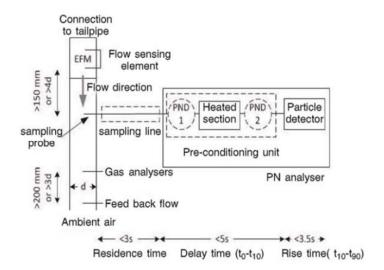
The PN analyser shall be connected to the sampling point via a sampling probe which extracts a sample from the centreline of the tailpipe tube. As specified in paragraph 3.5. of Annex 4, if particles are not diluted at the tailpipe, the sampling line shall be heated to a minimum temperature of 373 K (100  $^{\circ}\text{C}$ ) until the point of first dilution of the PN analyser or the particle detector of the analyser. The residence time in the sampling line shall be less than 3 s.
