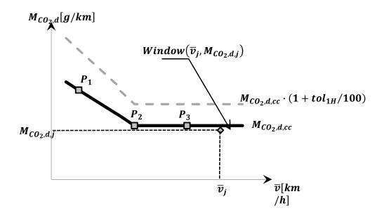
4.4.1. Low, medium and high speed windows (for analysis with 4-phase WLTP)
