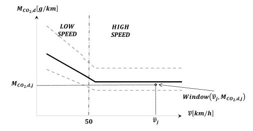
Figure A8/6-2. Vehicle CO<sub>2</sub> characteristic curve: low and high speed driving definitions (Illustrated for OVC-HEV vehicles)
