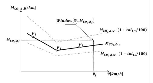
Figure A8/4: Vehicle CO<sub>2</sub> characteristic curve and tolerances for OVC-HEV vehicles
