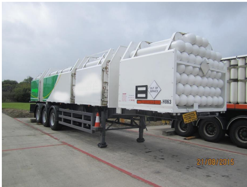
Battery vehicle constructed with seamless steel cylinders
