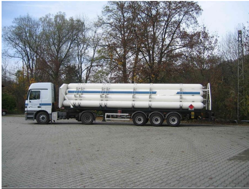
Battery vehicle constructed with seamless steel tubes
