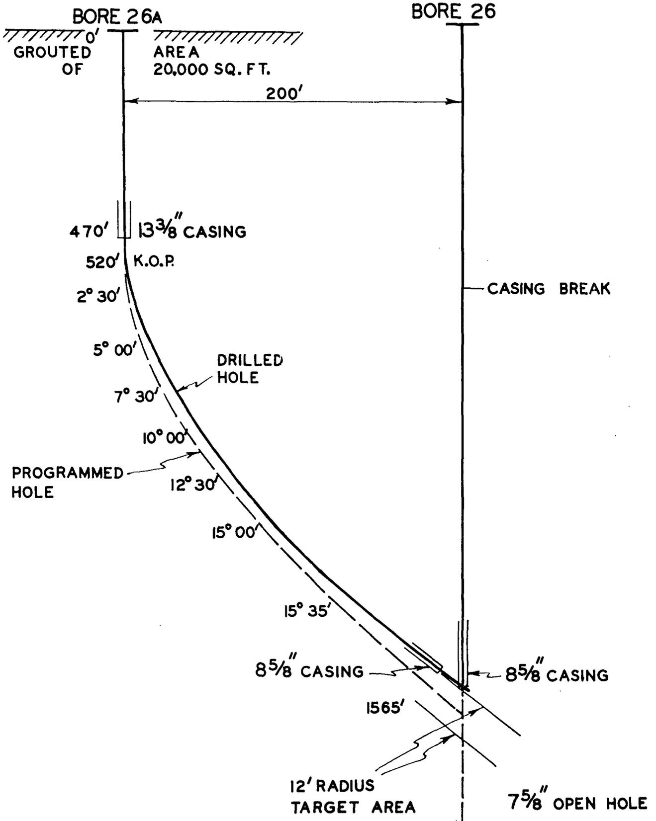
Figure 4. Deviated bore No. 26a
