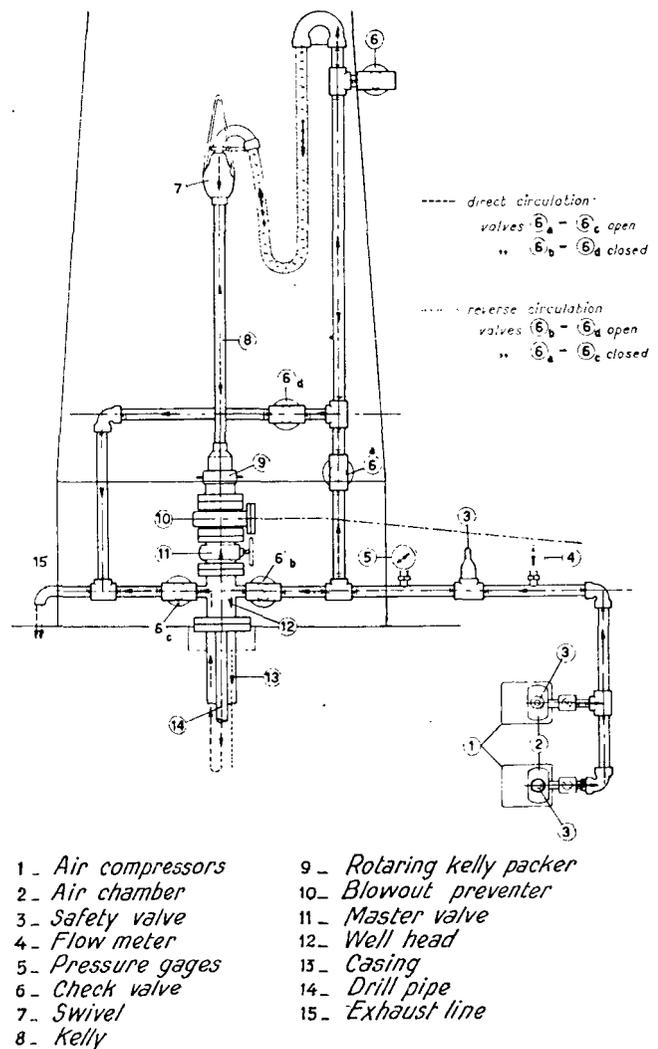
Figure 1. Surface equipment and stand-pipe arrangement for air drilling with direct and reverse circulation
