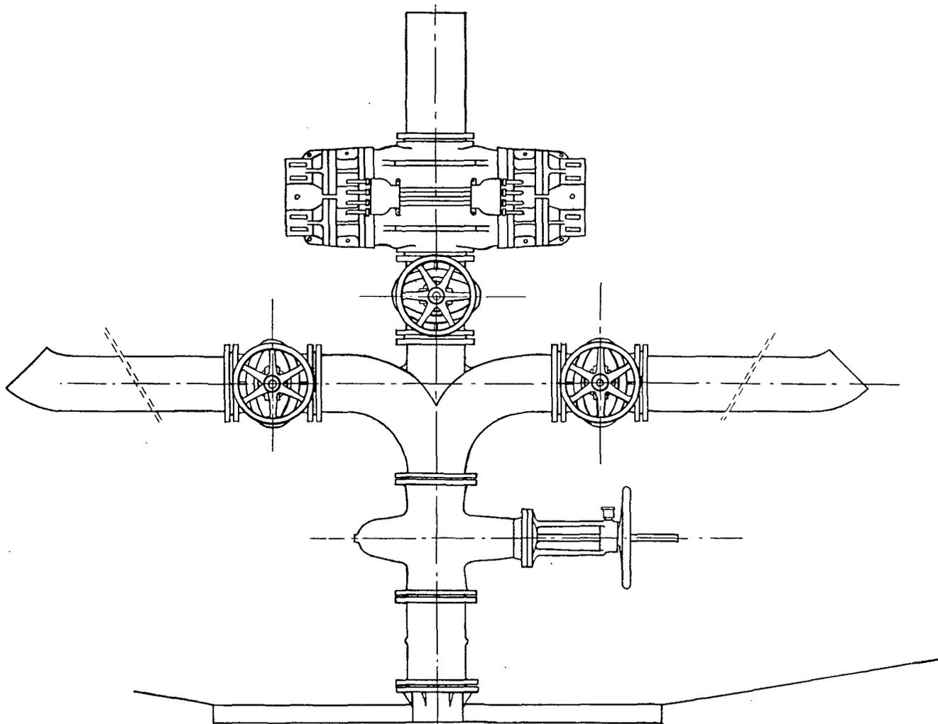
Figure 2. Christmas-tree with central valve and preventer at a natural-steam production well
