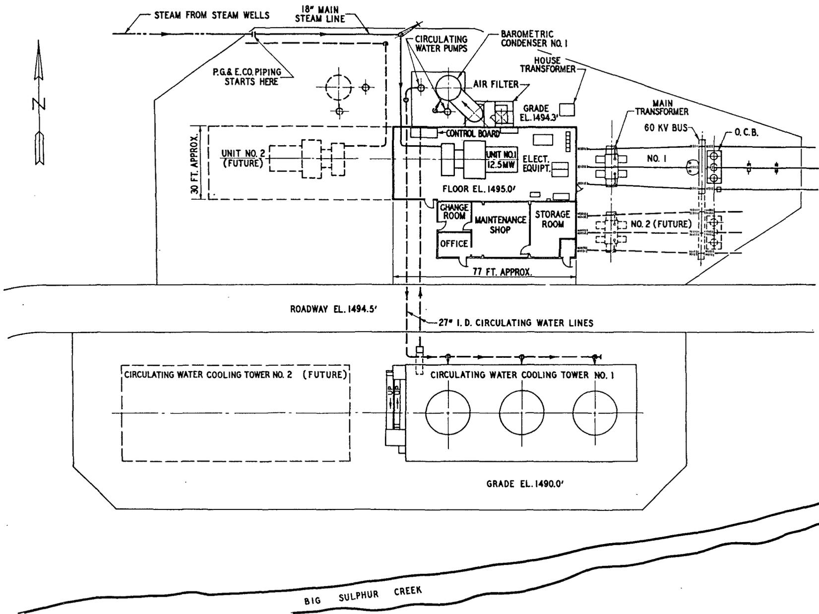
Figure 4. Plan of The Geysers power plant
