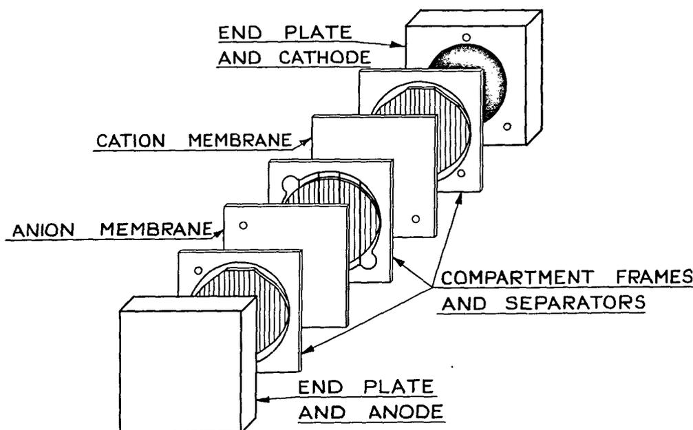
Figure 1. Exploded view of cell assembly
