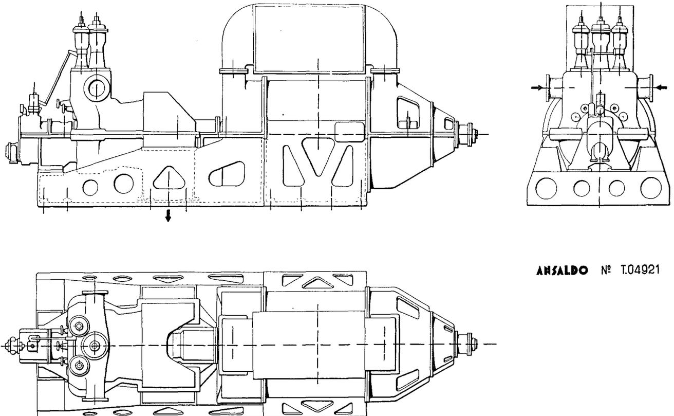
Figure 9. 5 000-6 000 kW turbine-generator set
