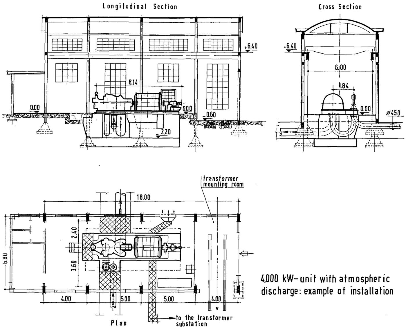
Figure 3. 4 000 kW unit with atmospheric discharge: example of installation
