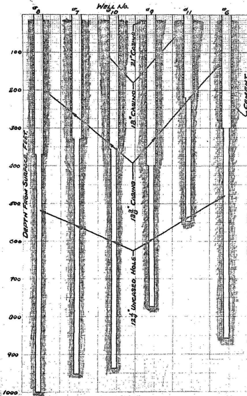
Figure 2. Outlines of well completion at The Big Geysers, California
