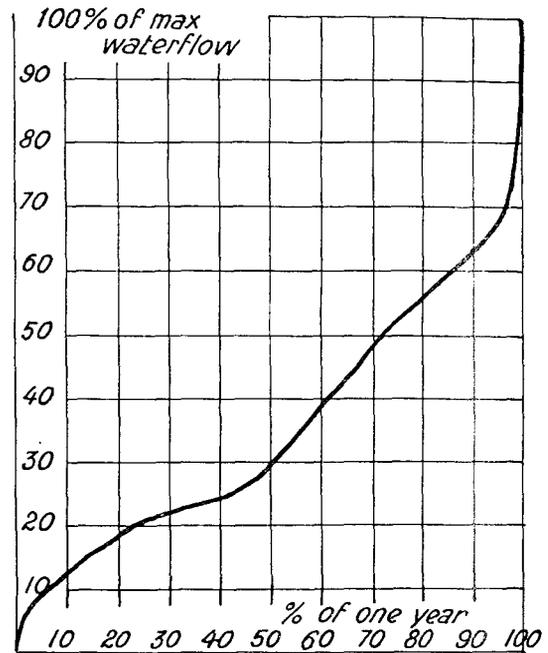
Figure 4. Reykjavik heating system: load duration curve
