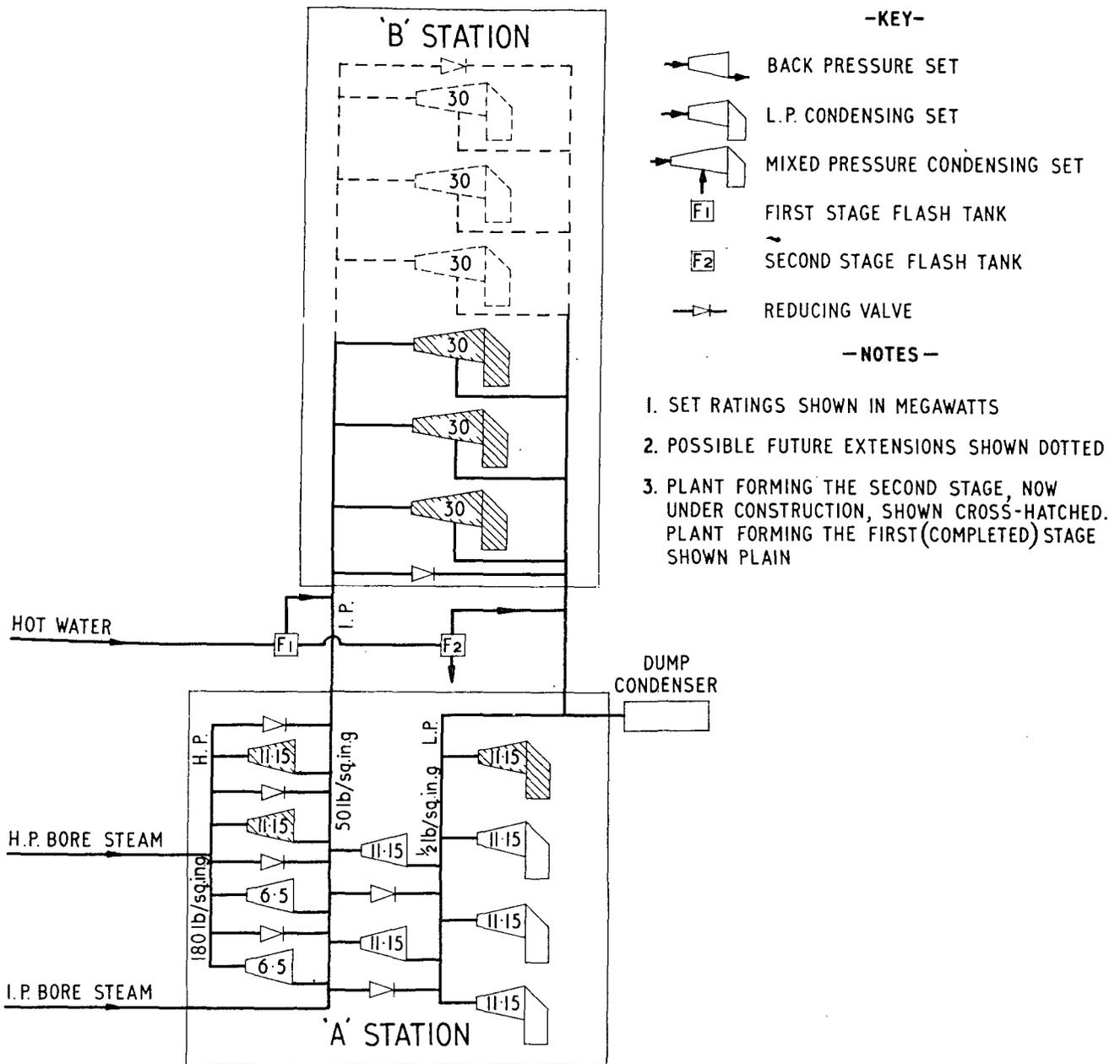
Figure 2. Arrangement of generating plant
