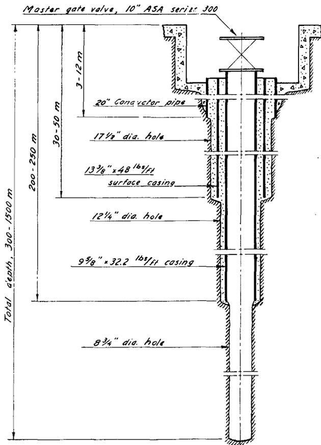
Figure 4. Drilling and casing programme —natural steam areas
