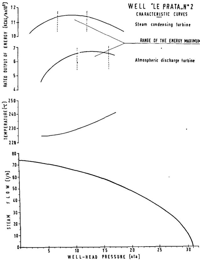
Figure 1. "Characteristic curves" of well "Le Prata 2"
