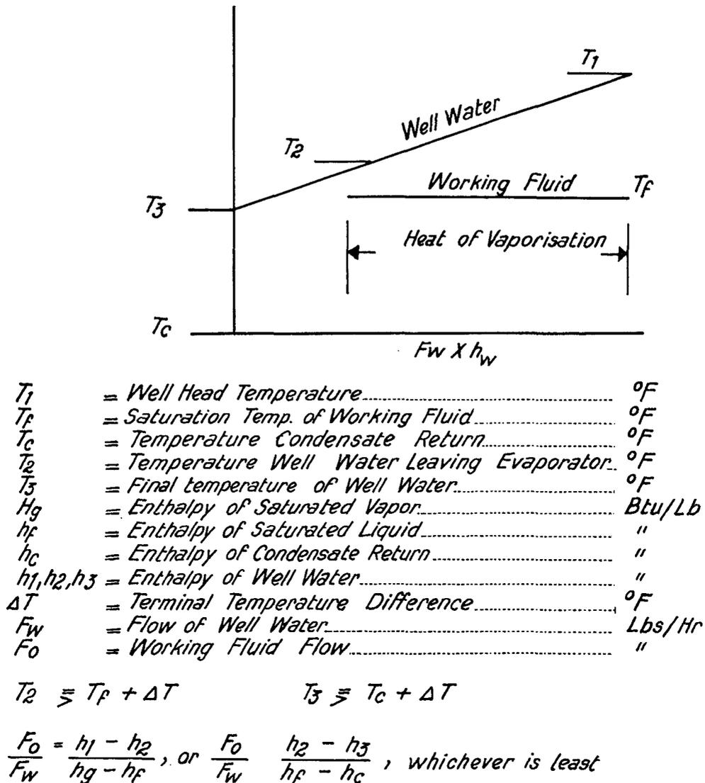
Figure 6. Heat exchange cycle
