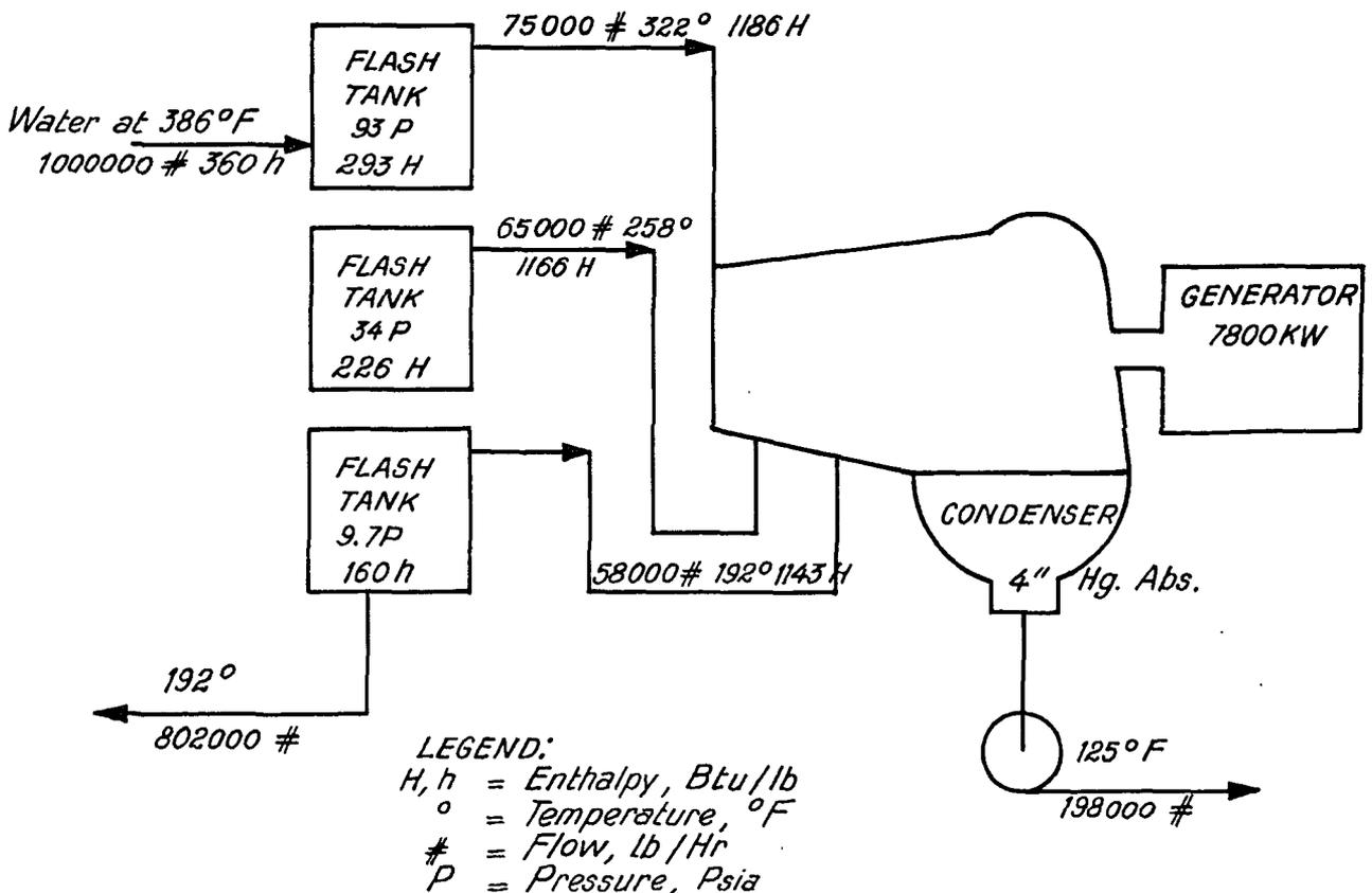
Figure 3. Multiple flashing cycle for geothermal application
