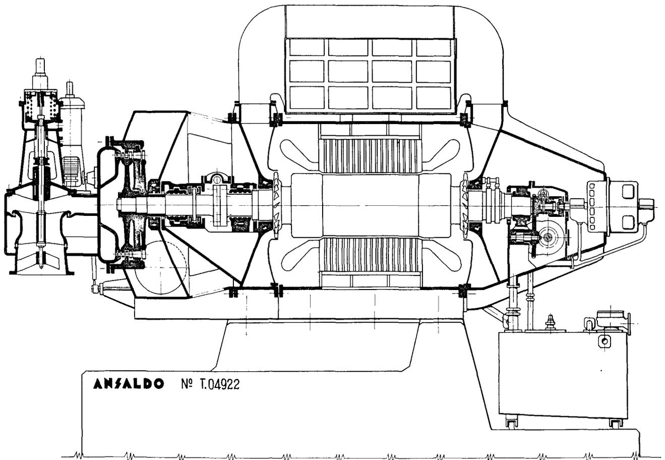
Figure 3. Cross-section of a 3 000-3 500 kW turbine-generator set
