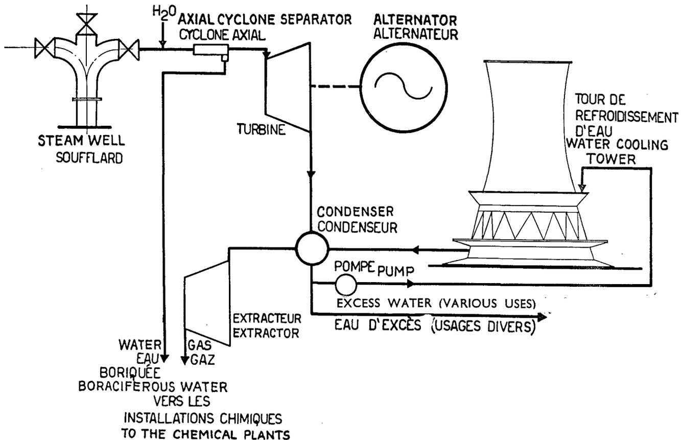
Figure 4. Power plant with steam scrubbing (scheme 4)
