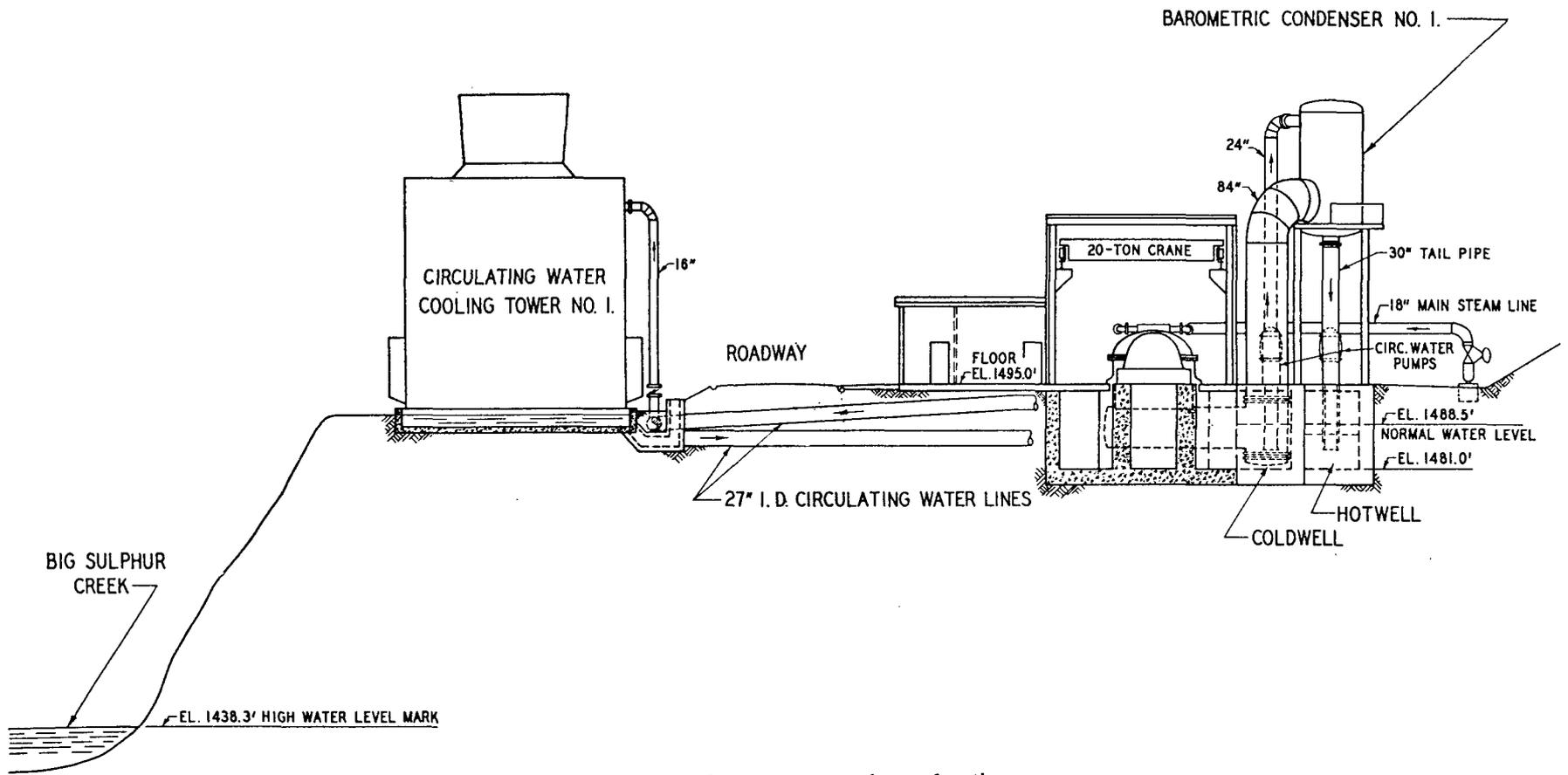
Figure 5. The Geysers power plant: elevation
