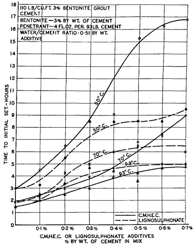
Figure 4. Setting times v. additive proportion for cement/bentonite slurries
