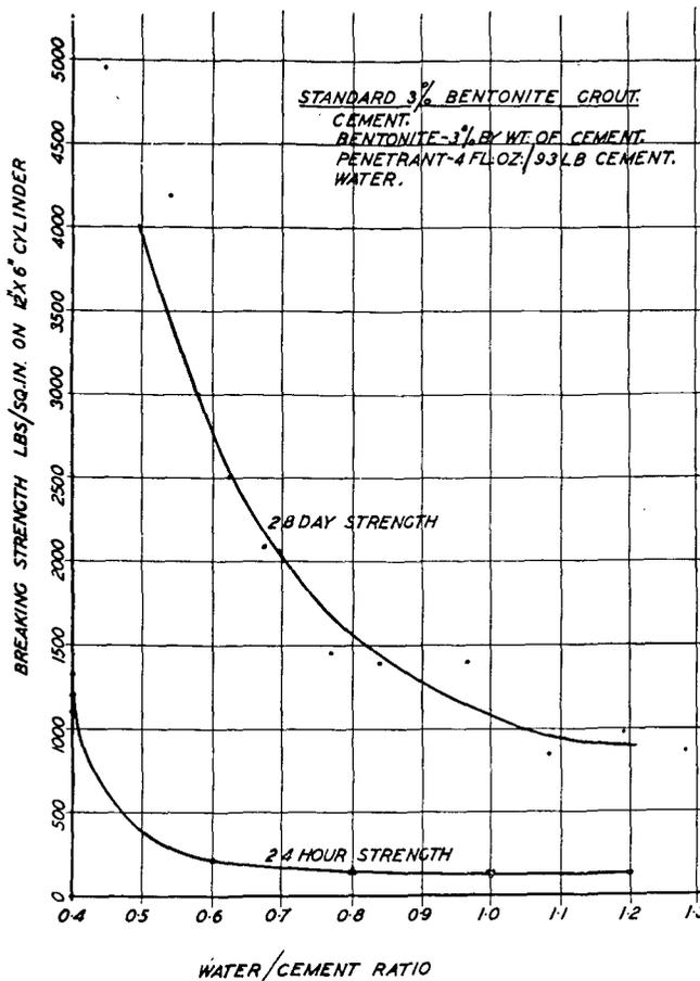
Figure 6. 24-hour and 28-day strengths of N.Z. cement normal slurries
