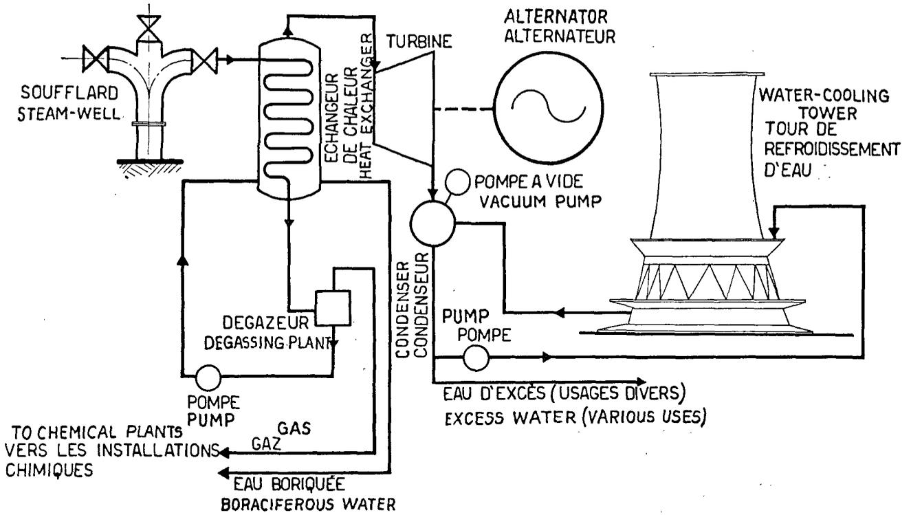
Figure 2. Pure-steam condenser power station (scheme 2)
