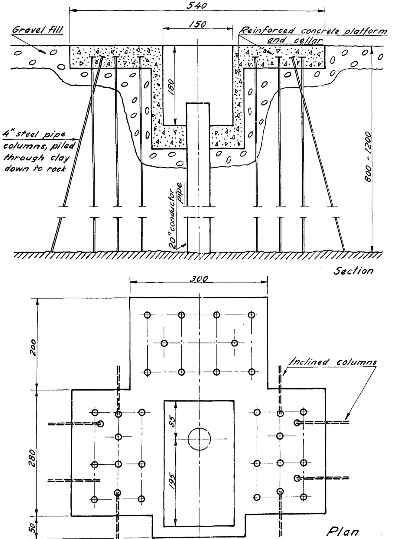
Figure 3. Foundation for rotary drilling equipment at Krysuvik, Iceland
