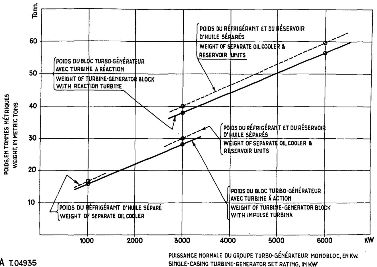
Figure 10. Weight diagram for turbine-generator sets
