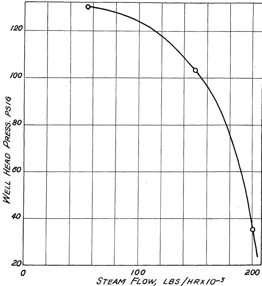
Figure 3. Thermal No. 11 full flow test, 16 Nov. 1960
