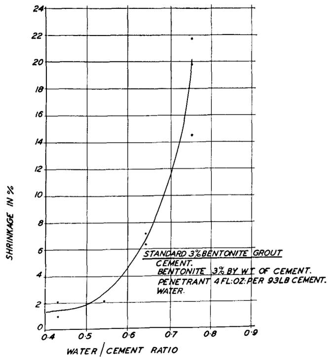
Figure 2. Shrinkage v. water/cement ratio for normal N.Z. cement slurries
