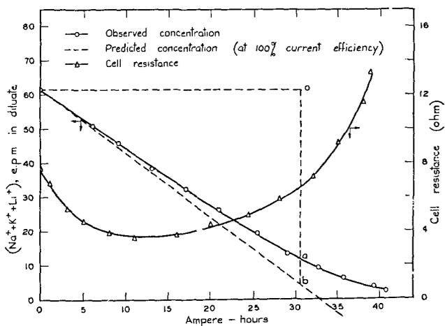
Figure 3. Current efficiency and cell resistance changes in desalting of bore water
