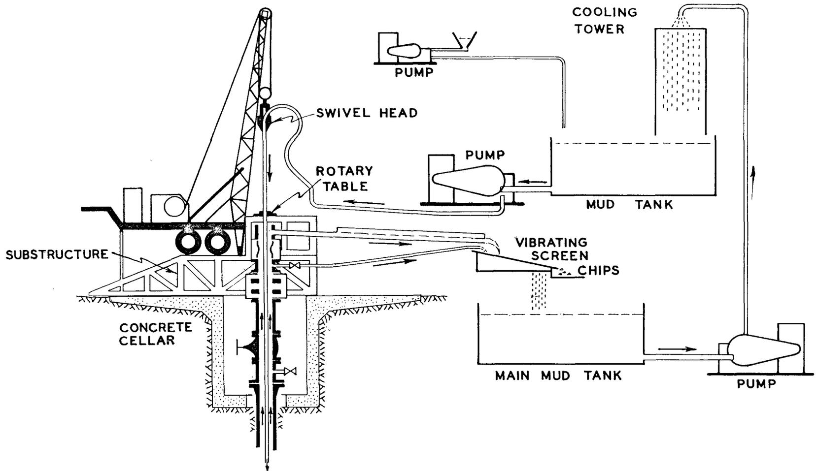
Figure 2. Typical rig and circulation layout
