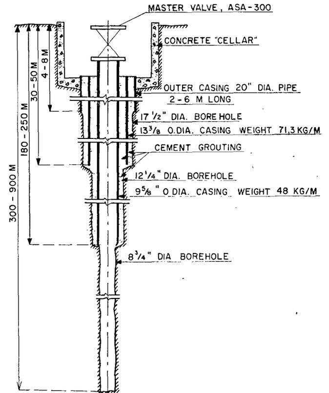
Figure 4. Steam wells at Hveragerdi: typical arrangement
