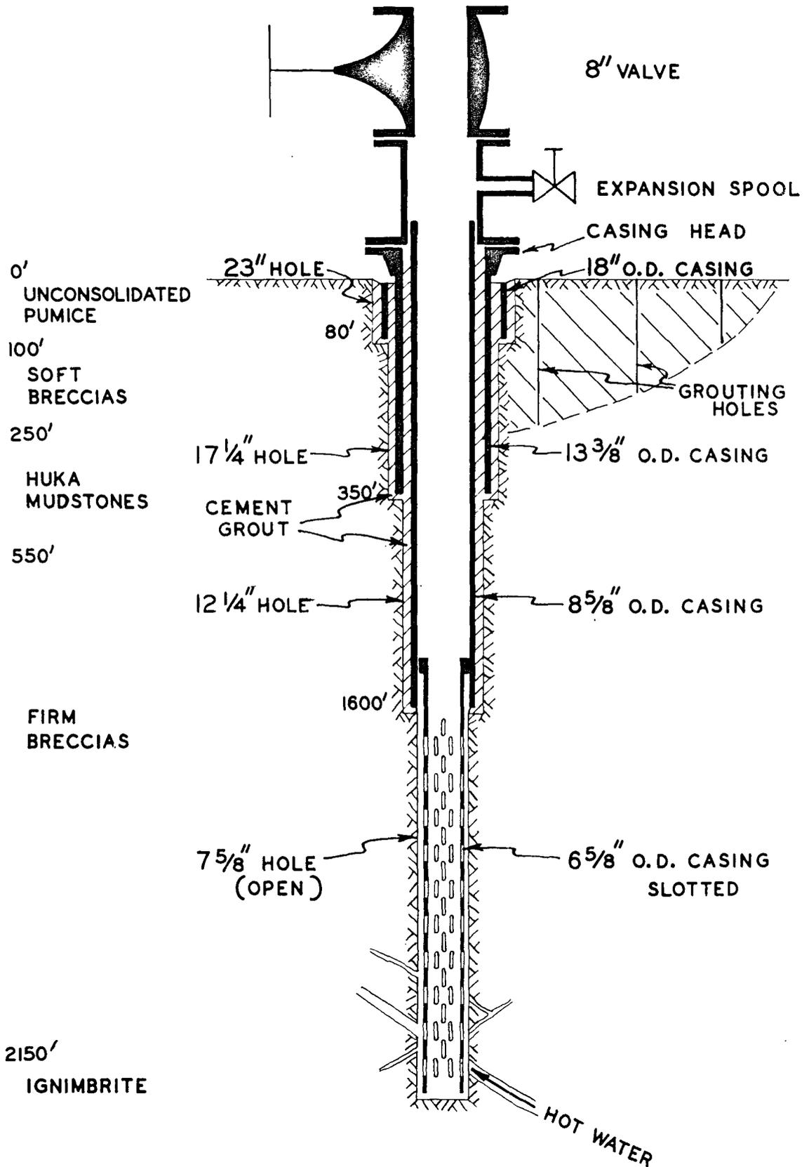
Figure 1. Casing layout and geological formations
