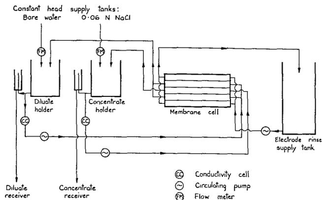
Figure 5. Schematic flowsheet for continuous desalting of bore water
