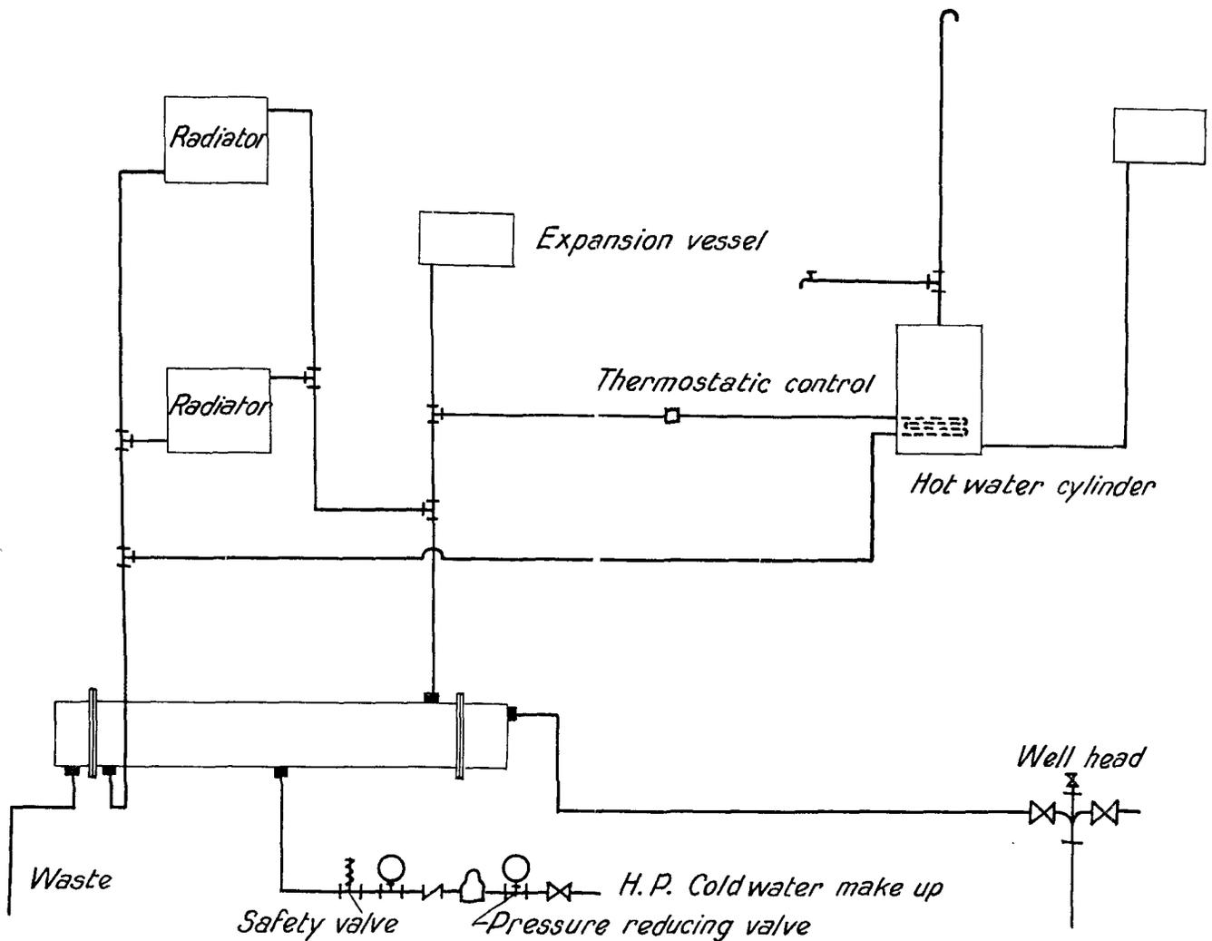
Figure 4. Line diagram of closed system
