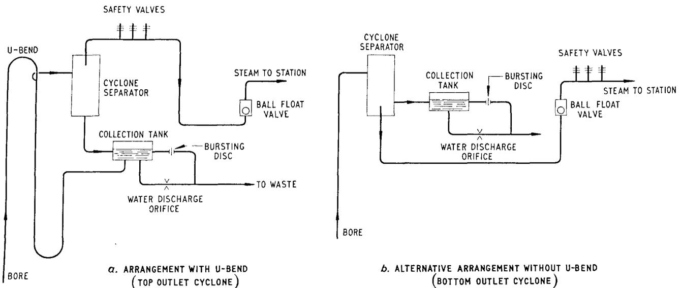
Figure 3. Diagram of wellhead equipment
