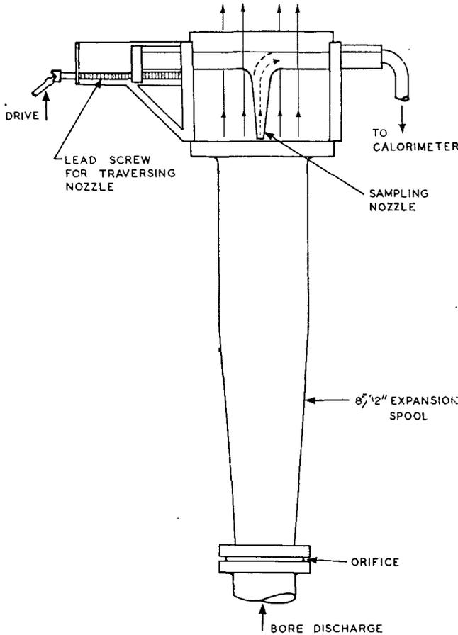
Figure 2. General arrangement of steam sampler
