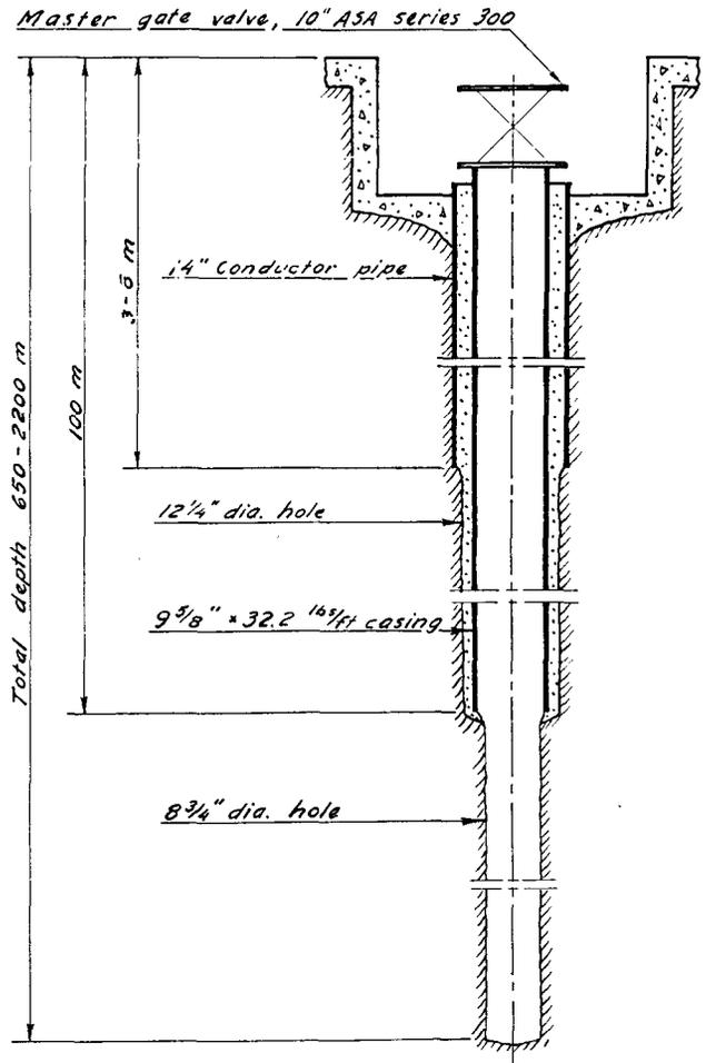
Figure 5. Drilling and casing programme —hot water areas
