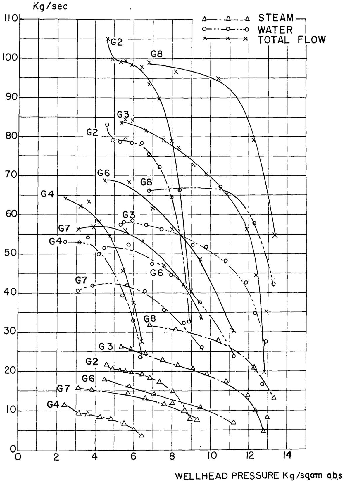
Figure 2. Flow characteristics of steam wells at Hveragerdi. The yield is measured at zero gauge (100°C)
