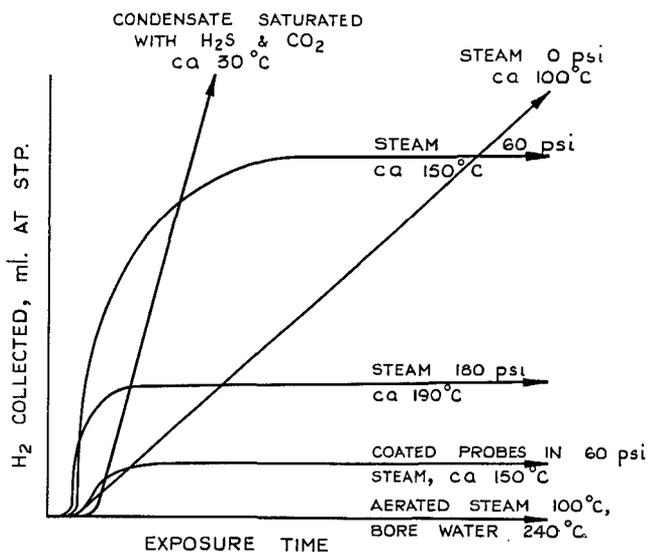
Figure 4. Typical probe results for clean and coated mild steel
