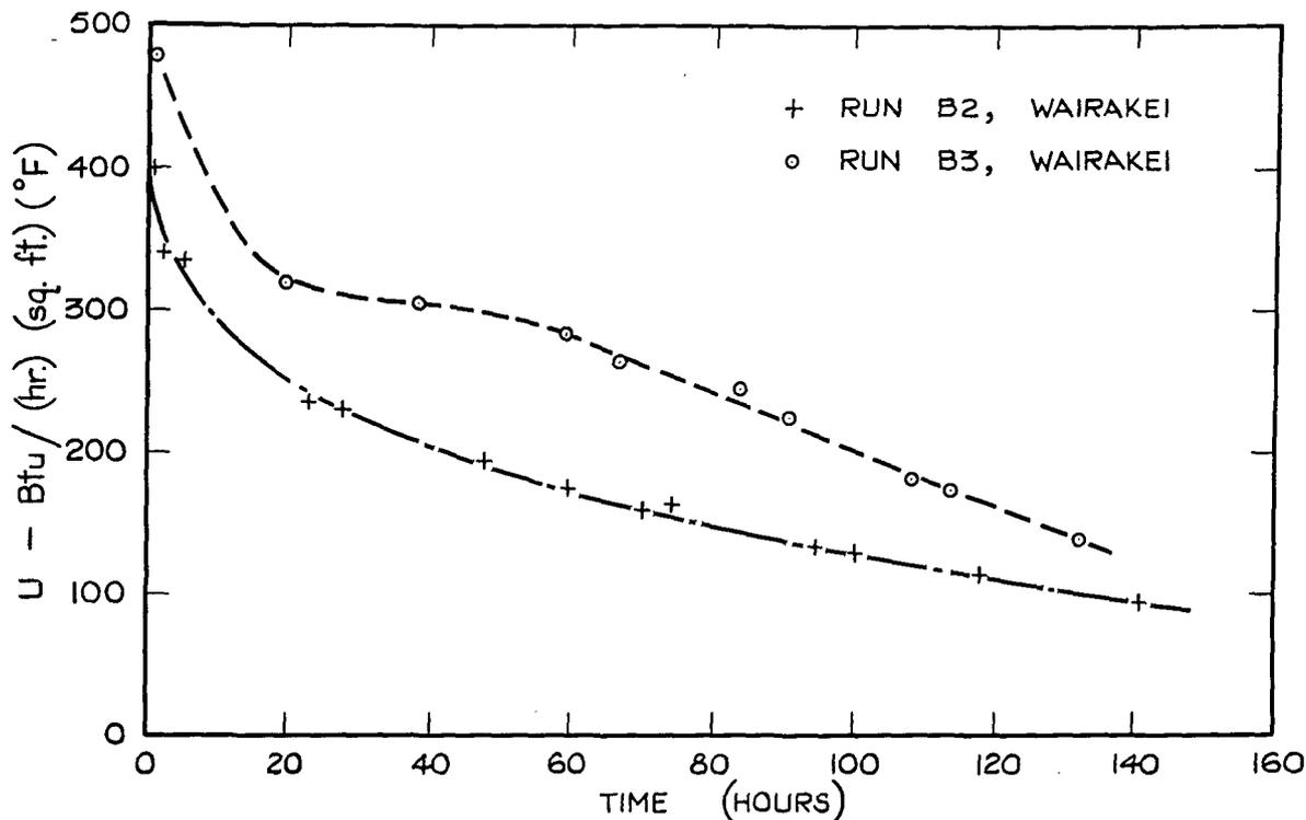
Figure 8. Effect of scale deposition on heat transfer coefficient
