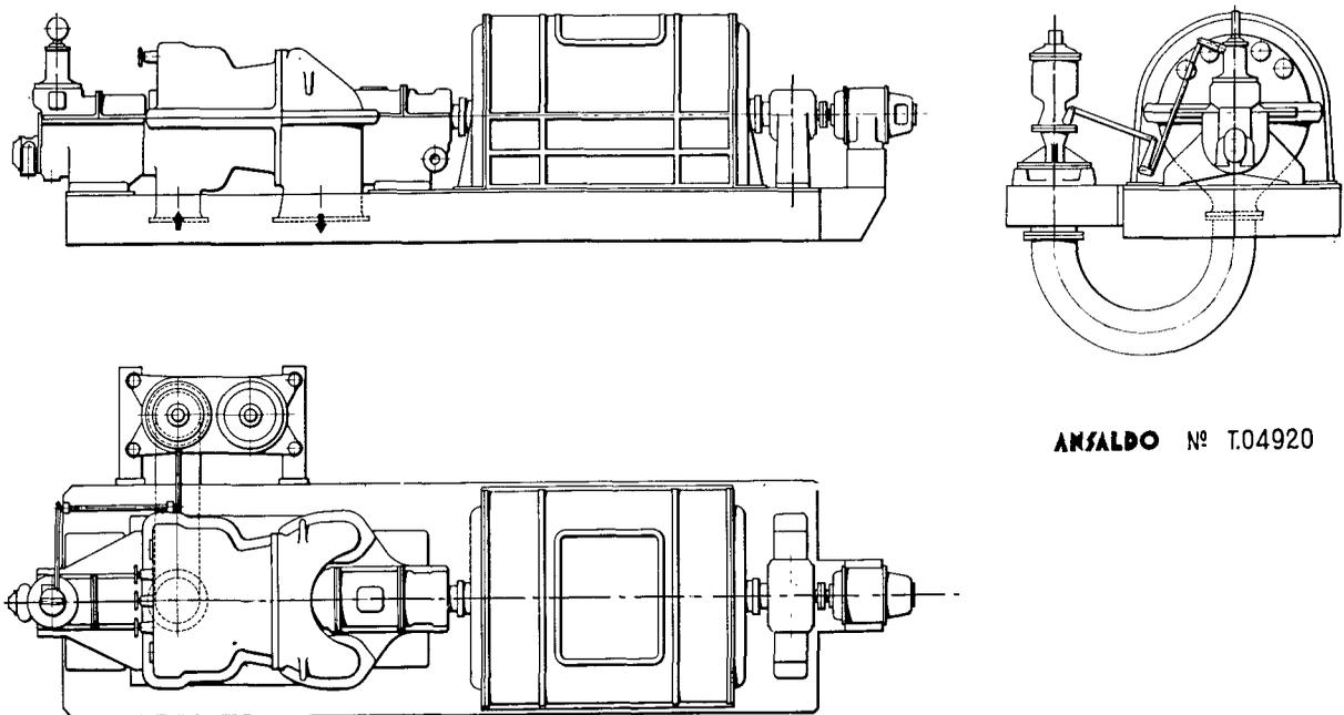
Figure 8. 3 500 kW turbine-generator set
