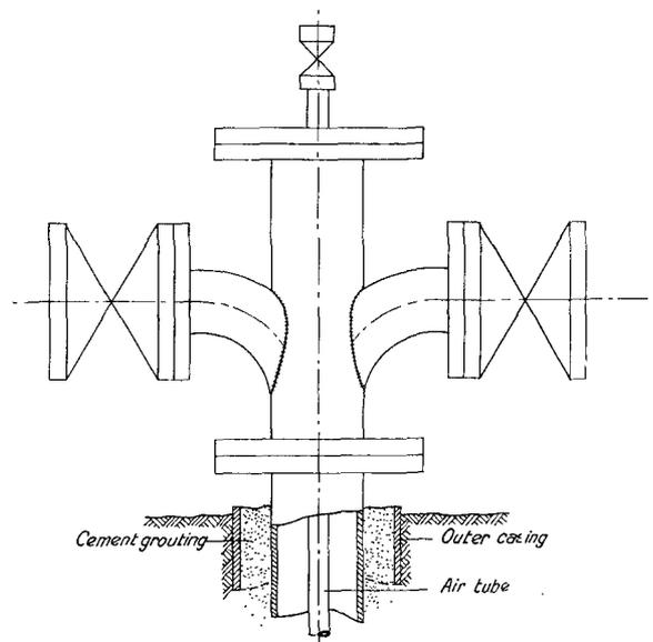
Figure 1. Diagrammatic representation of standard well-head
