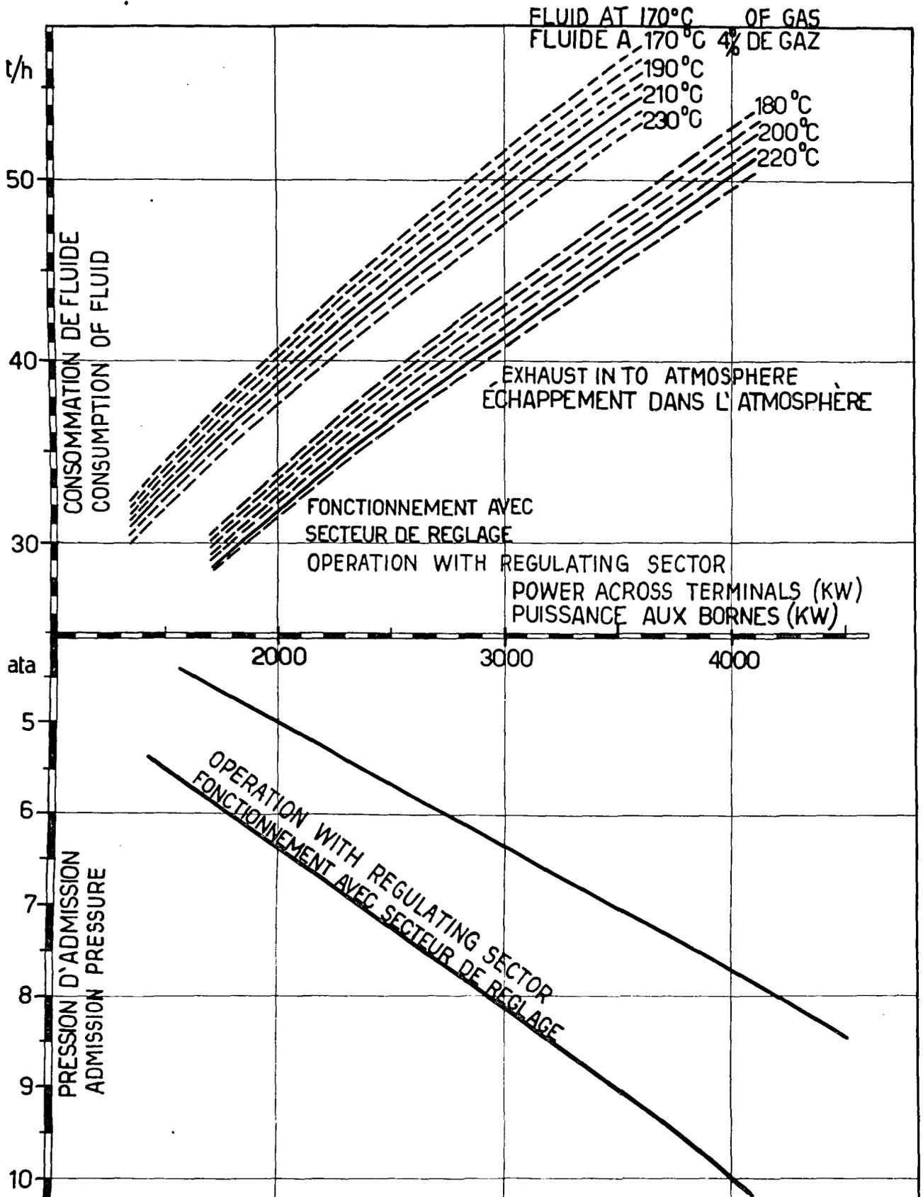
Figure 7. Consumption curves of 7-11 atm 4 500 kW unit
