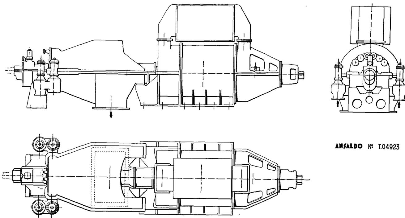
Figure 4. 7 000 kW turbine-generator set
