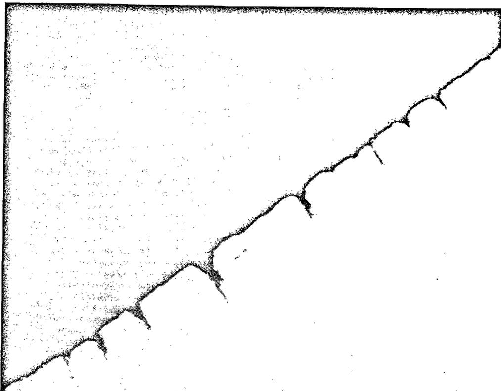
Figure 2. Metallographic section through surface fissures on a stress corrosion specimen
