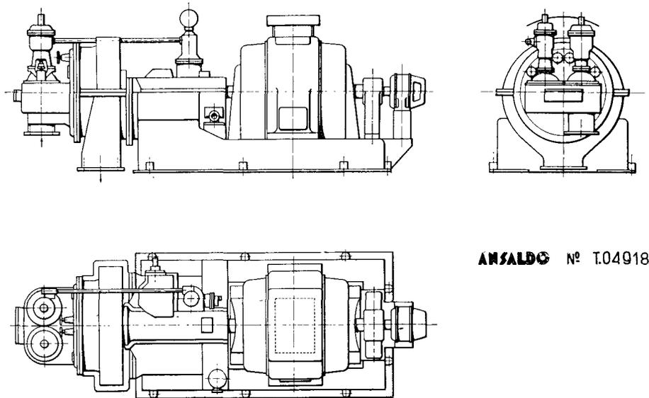
Figure 1. 900-1 250 kW turbine-generator set
