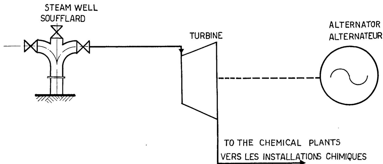
Figure 1. Natural-steam free-exhaust power station (scheme 1)
