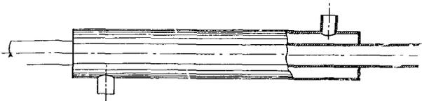
Figure 2. Simple tube and jacket exchanger
