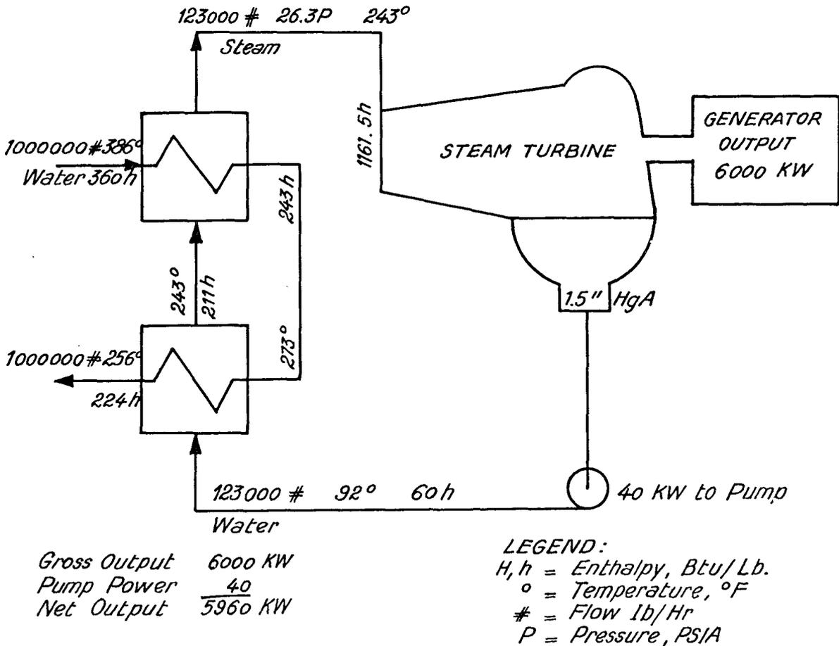
Figure 5. Heat exchange steam cycle for geothermal application
