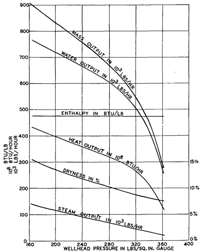
Figure 3. Output curves for bore 81 (a typical large output bore)
