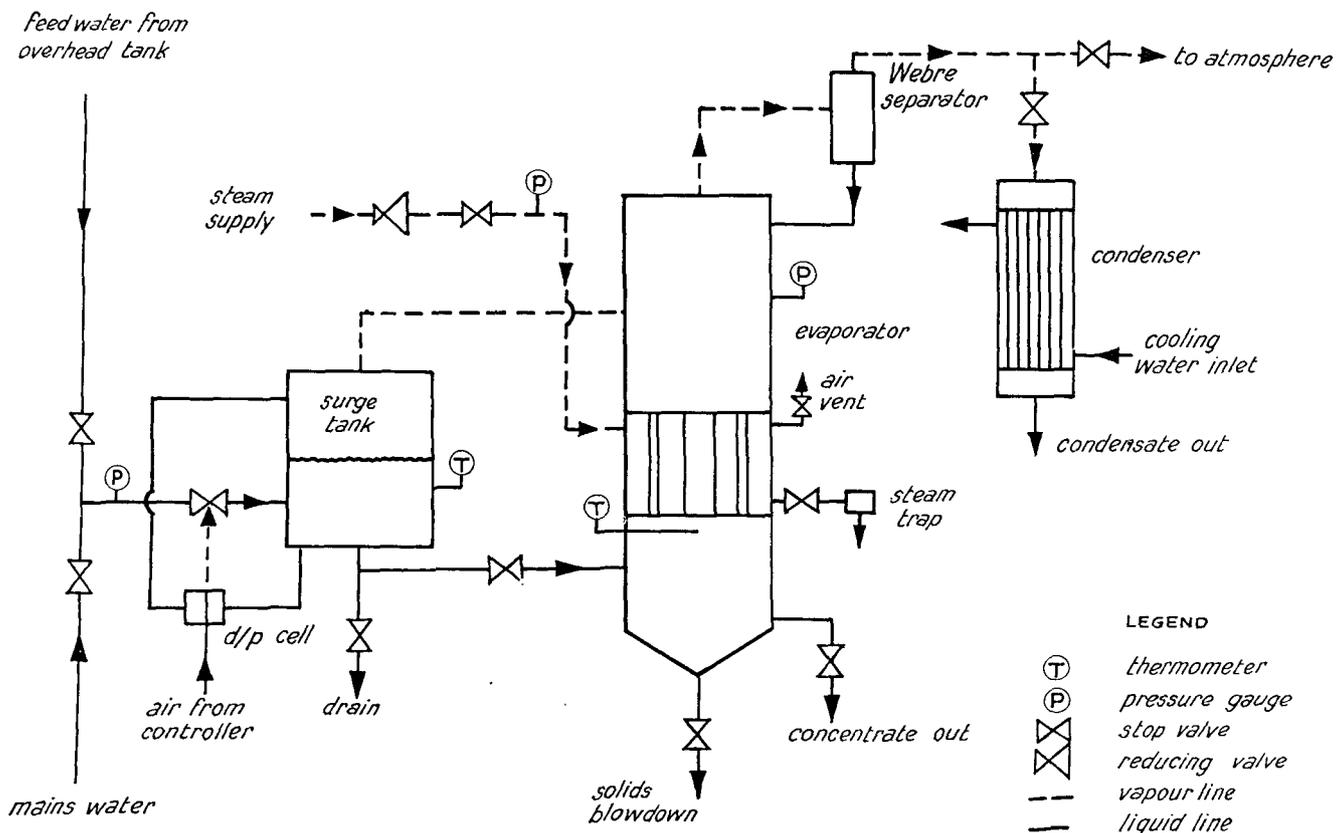
Figure 7. Sketch of evaporator layout
