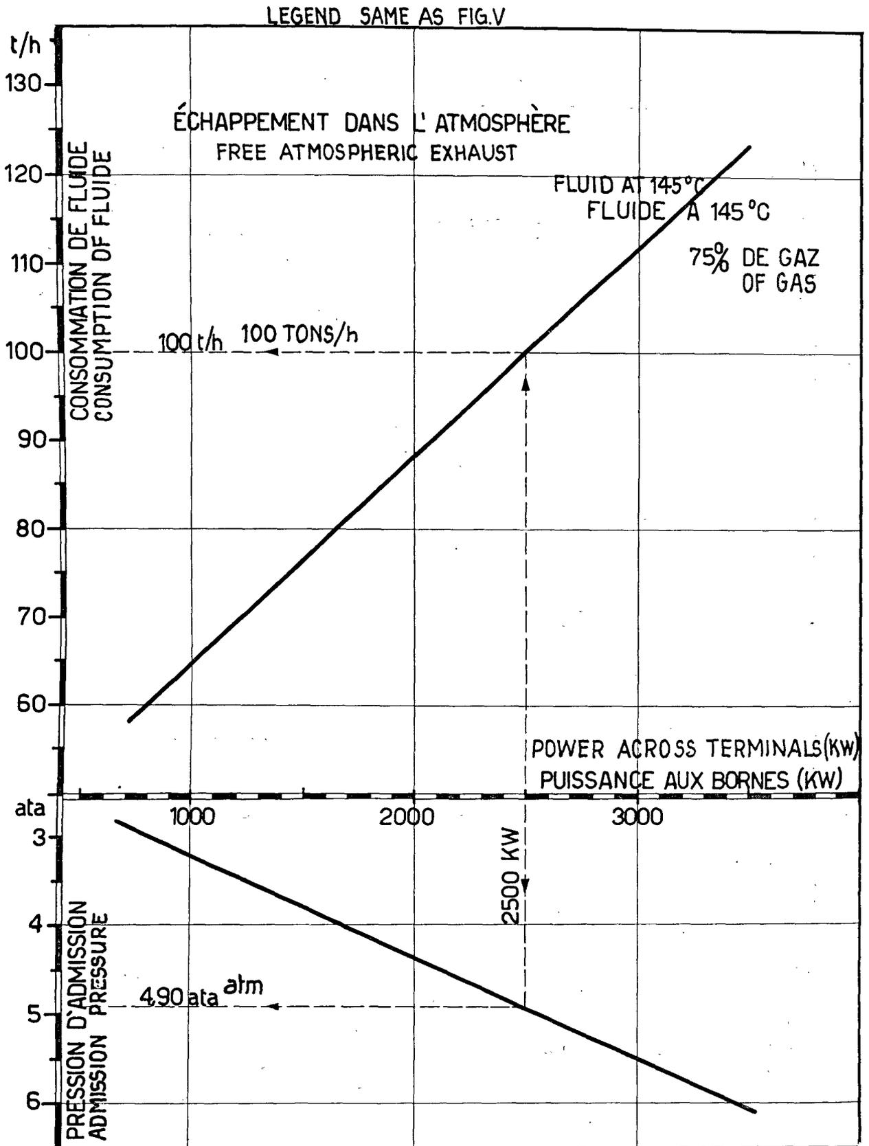
Figure 6. Consumption curves of 3 500 kW unit
