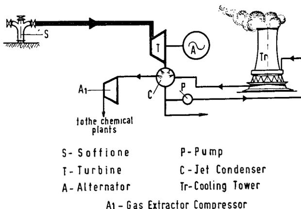
Figure 7. Condensation cycle with direct steam inlet
