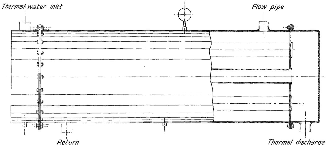
Figure 3. Simple form of all-welded heat exchanger
