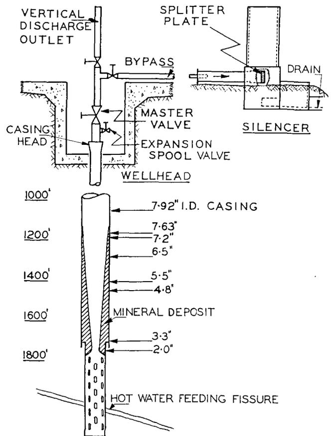
Figure 3. Typical mineral deposit build-up in a bore casing
