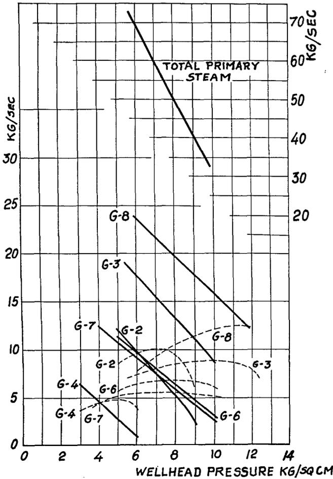
Figure 3. Primary and secondary steam fractions obtainable from the steam wells
