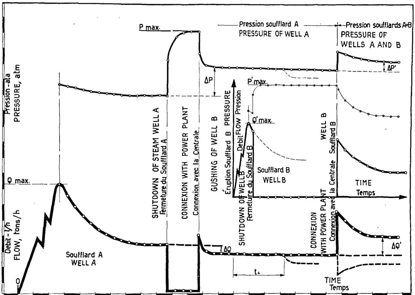
Figure 14. Operation of steam wells with shutdown equipment
