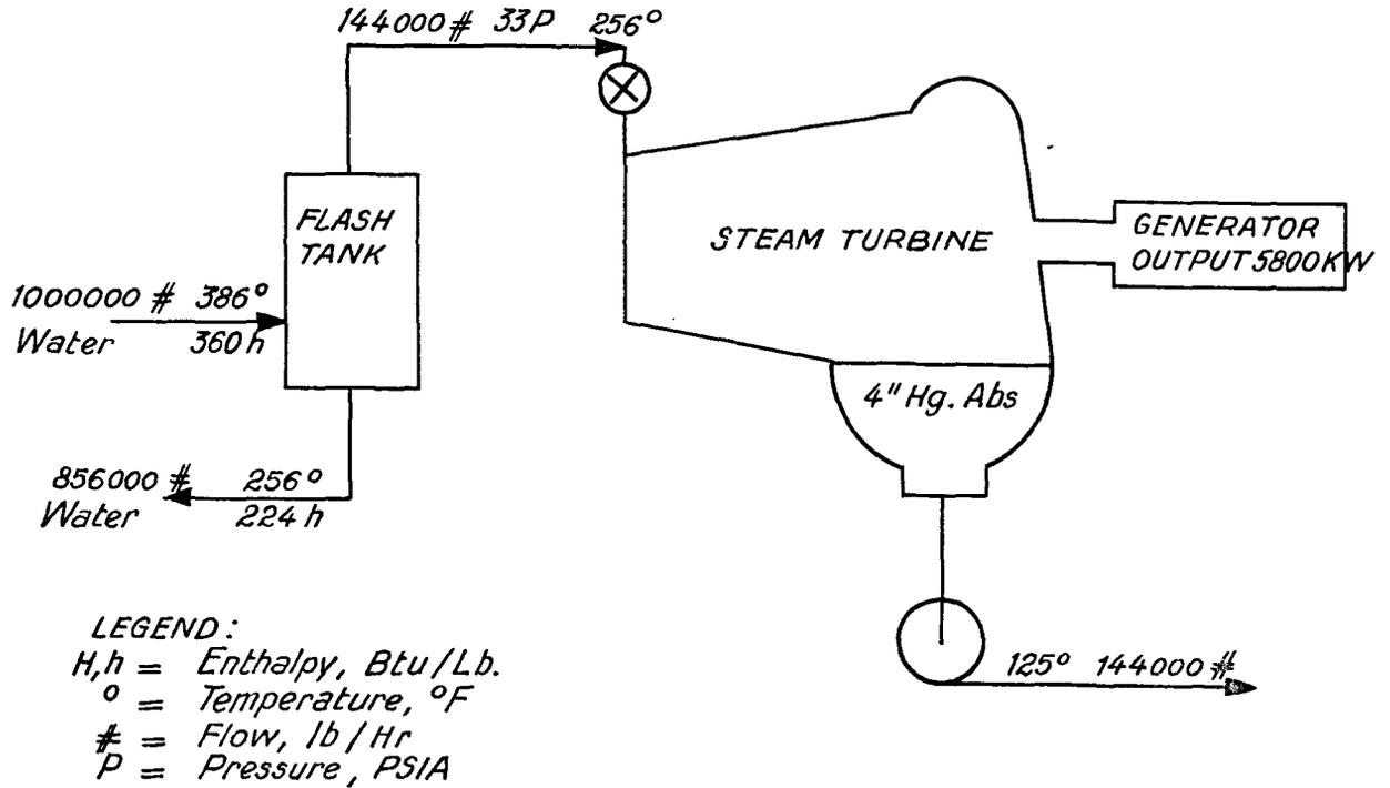
Figure 1. Simple flashing cycle for geothermal application
