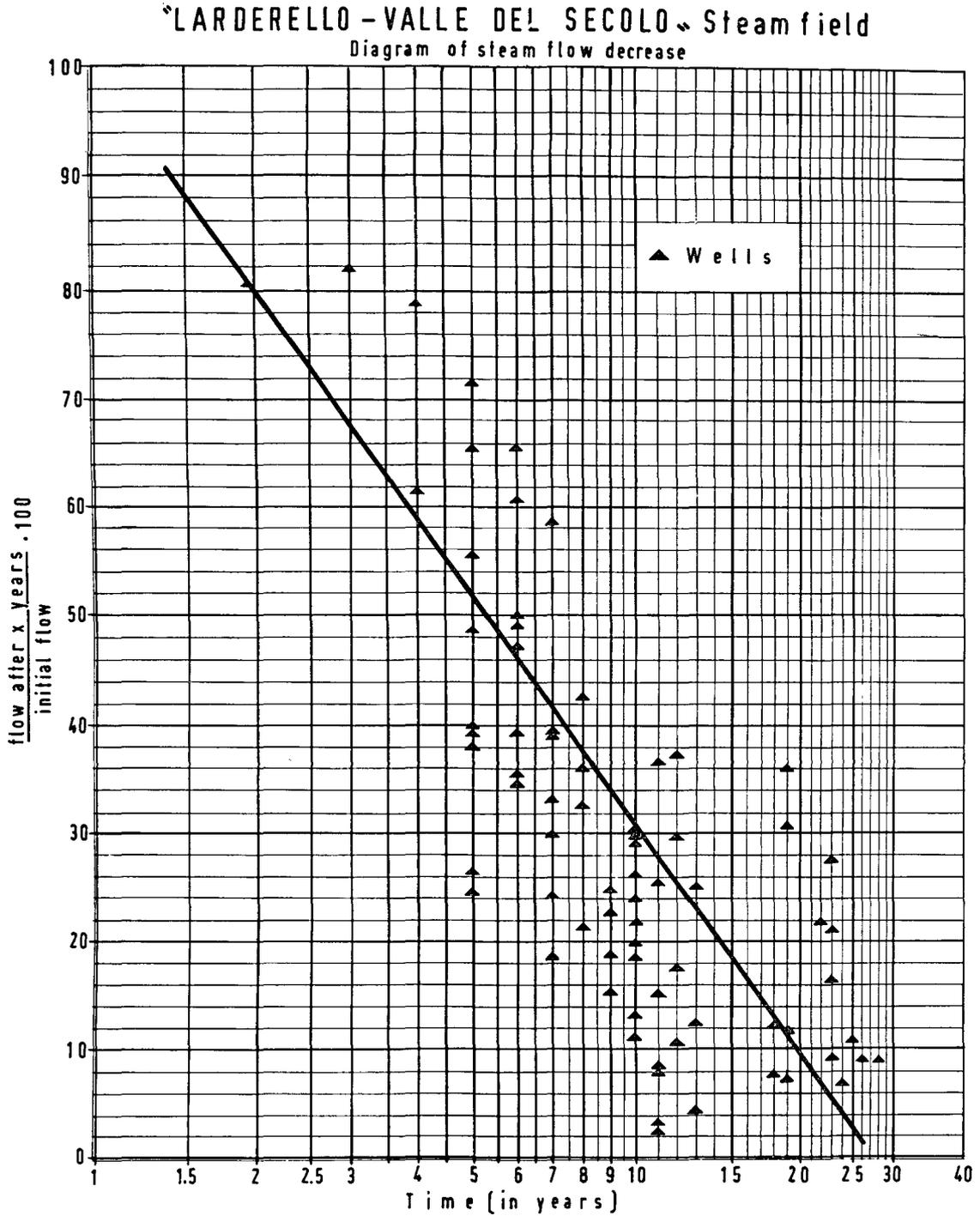
Figure 10. "Larderello—Valle del Secolo" steam field — steam decrease curve
