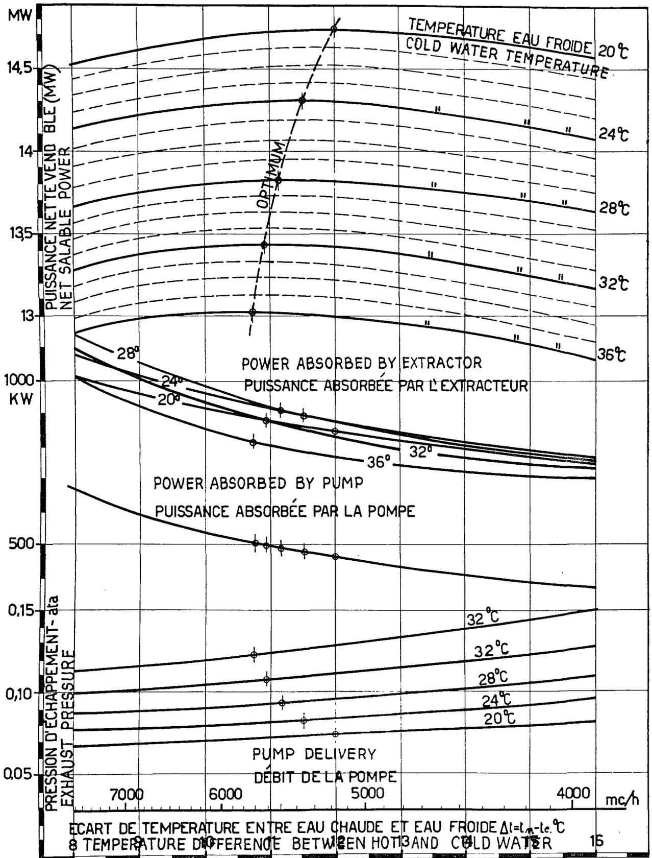
Figure 11. Finding the optimum for the auxiliaries of a natural steam unit
