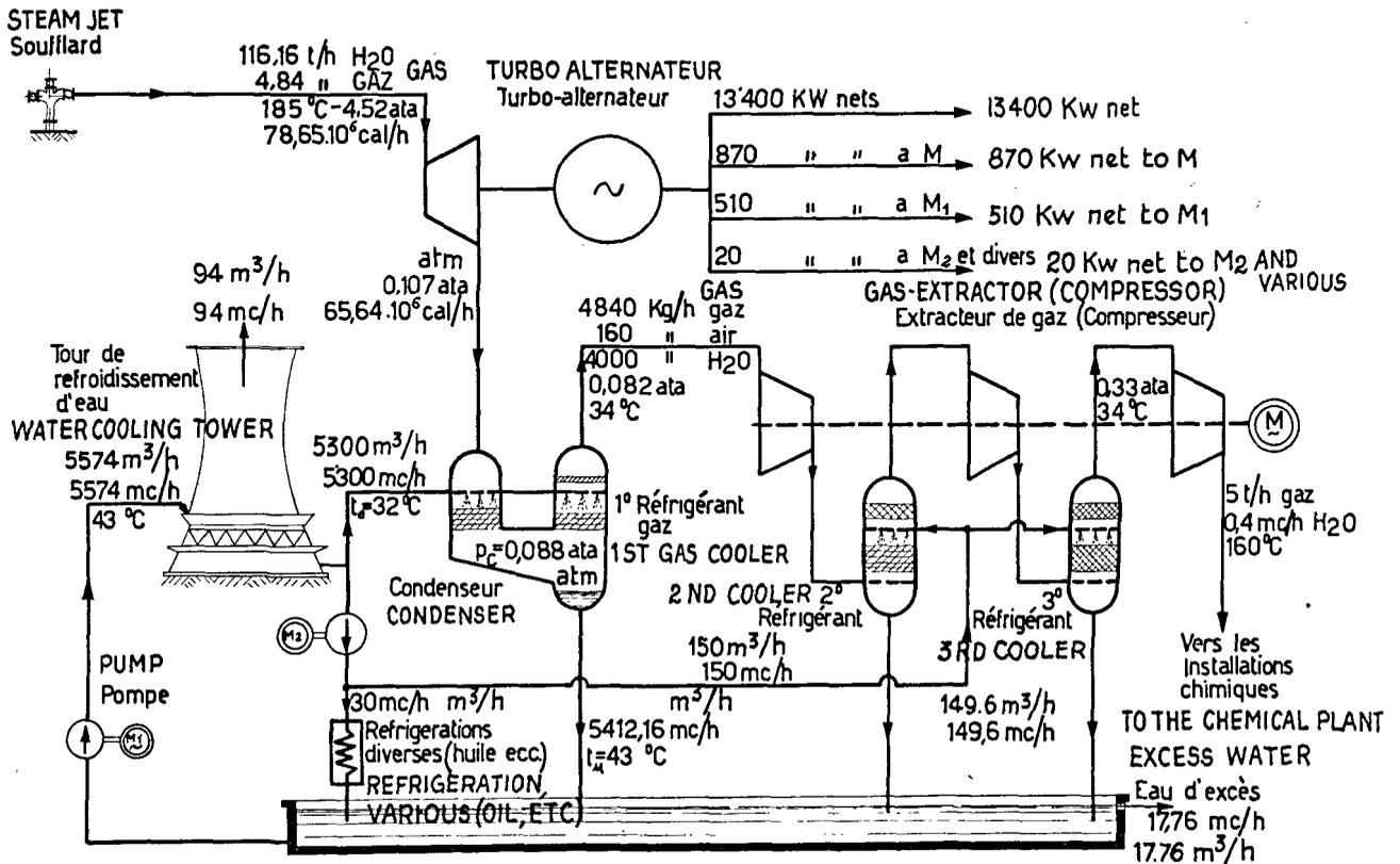
Figure 3. Natural steam condensing power plant (scheme 3)
