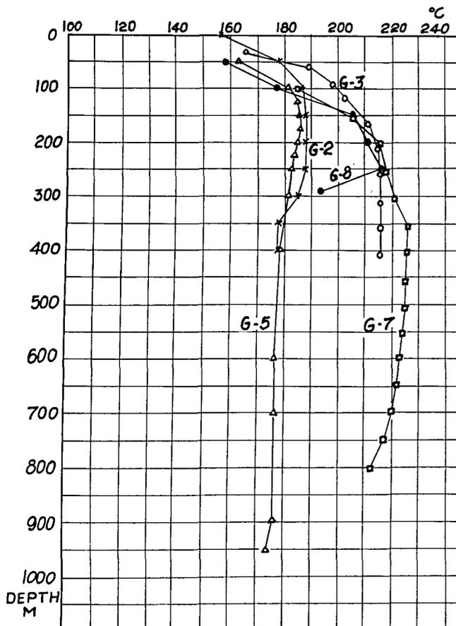
Figure 5. Measured temperatures in steam wells at Hveragerdi
