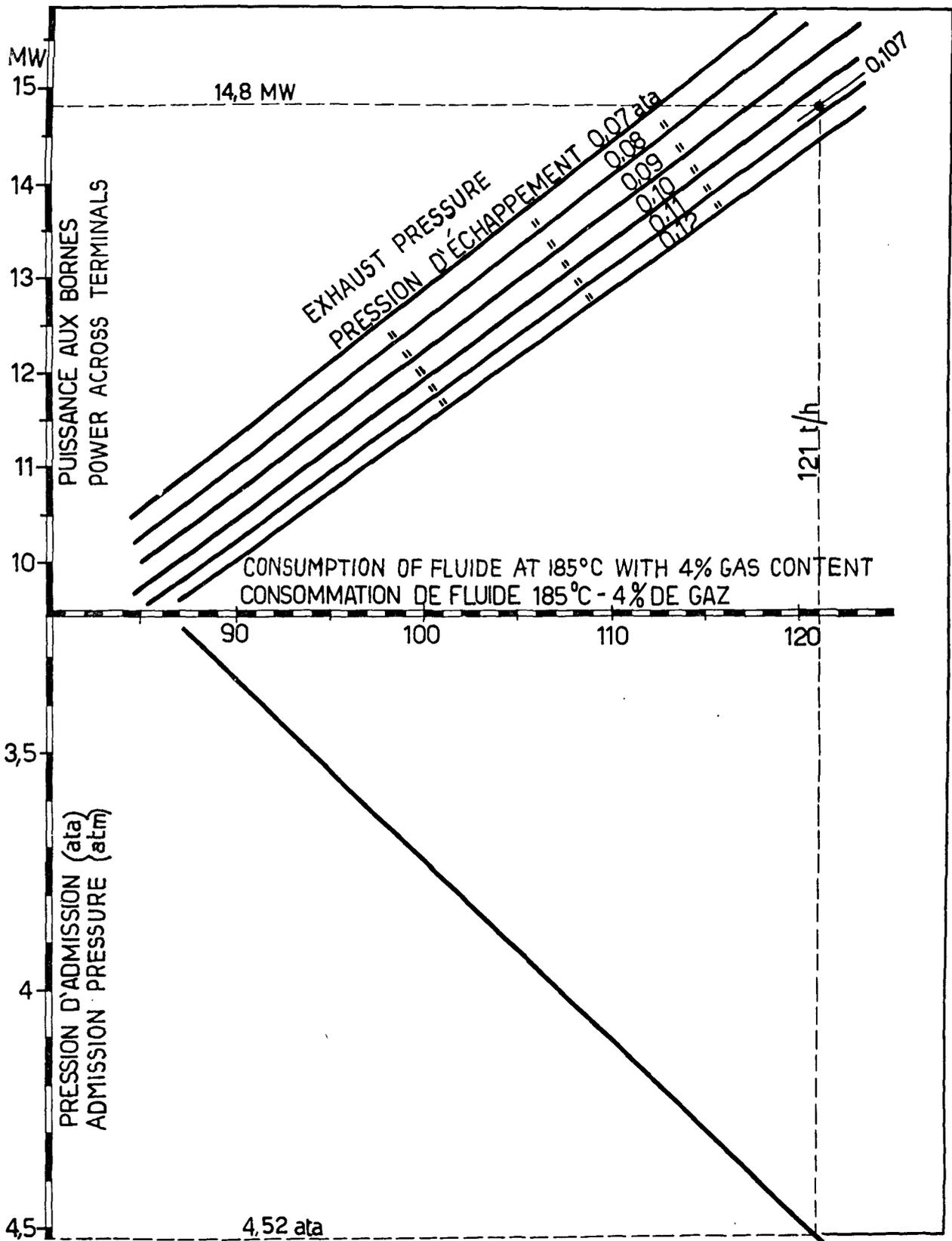
Figure 8. Consumption curves of 1 500 kW unit
