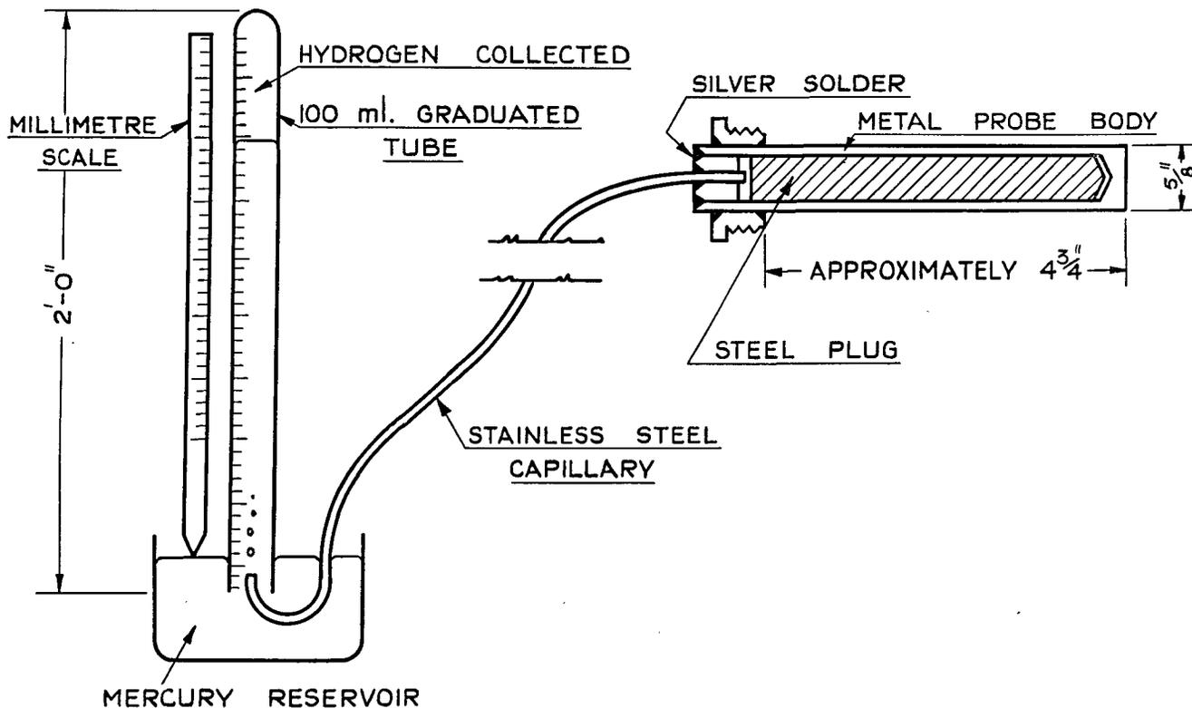
Figure 3. Hydrogen probe
