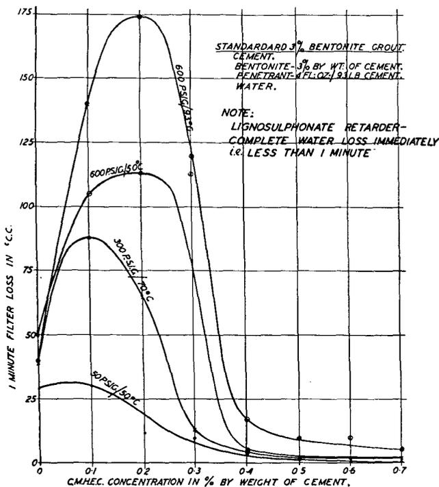
Figure 5. Water loss v. proportions for normal and L.W.L. additives with N.Z. cement slurries
