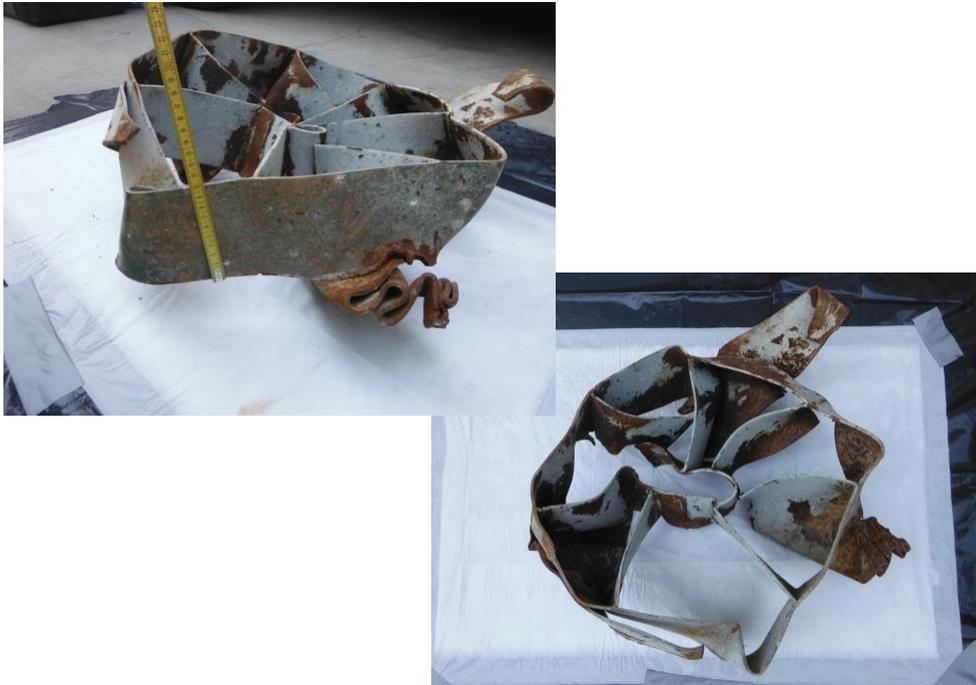
12. 01SDS(B) is a large corroded and deformed metal object. Despite the corrosion, it is still possible to see layers of dark green and grey colour. It is also possible to see a smaller inner ring in the middle, linked by seven metal parts to a larger, outer ring. Four of the parts that are linking rings are rectangular. The other three are much larger and triangular. The spacing between the three parts, in addition to indications on the rings, point to one missing larger triangular part.
