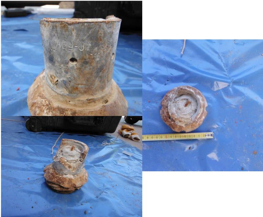
8. 09SDS is a heavily deformed and damaged metal object. On the both sides threads are visible. This part also bears visible markings which point to a universal bomb fuse. The fuse has been activated and does not contain explosive material. This device is normally electrically armed, heat resistant, and can function as point detonating or with delayed action. It is used on a large number of aerial bomb types by numerous nations.
