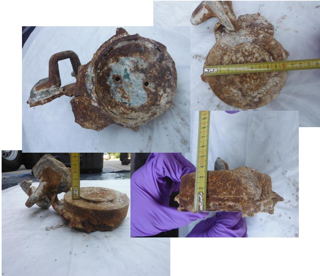
17. It is heavily corroded however, on the lid of the circular part, and on the welding of the hook-shaped part it is possible to see traces of dark green paint. The circular part looks very similar to the circular part of sample 07SDS (see previously) and has very similar dimensions. The dimensions are therefore not repeated here.
