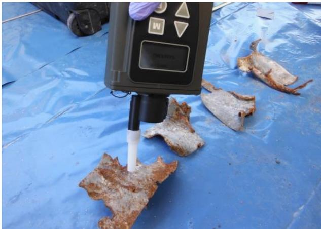
9. 10SDS comprises four smaller metal pieces. Less rust is visible than on the other items. Fragments are grey with sharp twisted parts and are made of thinner material than most of the other items. The deformations indicate that explosion has torn them off of a larger system. Although the flat lines on the sides, together with the general shape and thickness, indicate that these items could potentially be a part of the tailfin assembly, the exact origin of this part could not be determined.
