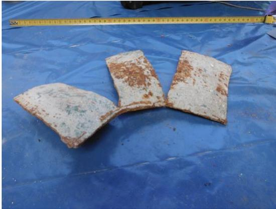
10. This item is moderately corroded metal part with visible dark green colour on the surface. It consists of three splintered parts still linked at one point. The thickness of material is approximately 5 mm; the length of individual pieces is approximately 180 to 200 mm, while the estimated total width of the linked part is approximately 320 mm.
