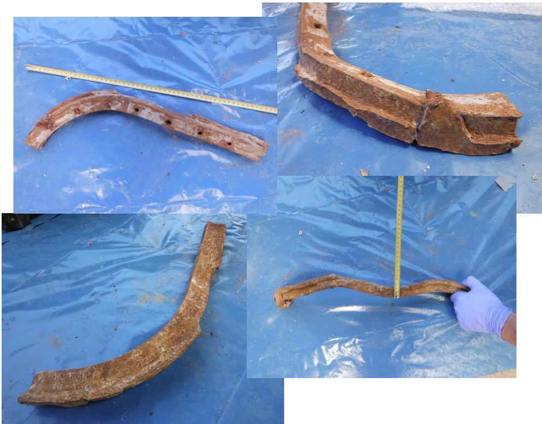
11. 12SDS is similar to a metal rail, approximately 550 mm long, with a square shaped cross section. It is heavily corroded with eight equally distributed holes visible on one side and traces of grey colour. Some of the holes still contain broken bolts inside. The width of the side with holes is approximately 30 mm, thickness is approximately 20 mm and the distance between two holes is approximately 65 mm. On one side there is an attached layer of metal, which is approximately 5 mm thick.
